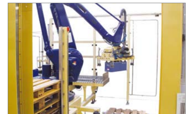
Flexible palletising: with the articulated robot.
